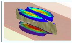
Iso-contours of HF induced formation shear damage in over/under-burden layers
