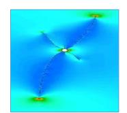
Frac propagation under the effect of wellbore stresses (plan view) (least compressive stress contours)
