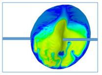
Proppant distribution inside a curving fracture (assuming gravity)
