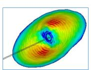
Fracture curving in 3D (contours showing aperture)
