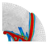
(c) Simulation subsequent to gross collapse through adaptive remeshing
