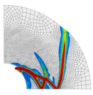
(b) Adaptive refinement in the zones of high shear strain localization
