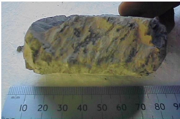
Fig. 3 – Blocky cavings recovered from extended-reach wells drilled at the Valhall field, indicative of bedding-parallel failure 13 .
